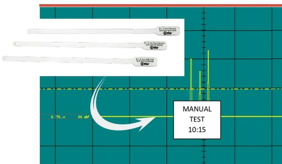
**AT 11:15 AND 12:15 THE METAL DETECTOR PERFORMS TWO AUTO-QC TESTS**, providing the previously recorded signal stimuli to the probe-emitter-receiver system and verifying the actual detection and product ejection (if applicable).
