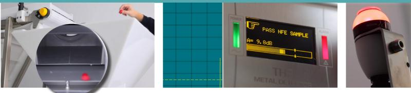
In addition to the AUTOTEST function, THS/21 and THS/MS21 detectors can be programmed so that **periodic verifications of the calibration are carried out automatically. This feature is called AUTO-QC<sup>®</sup> TEST**.
