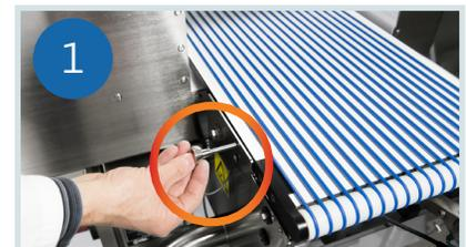
Remove the four locking pins
